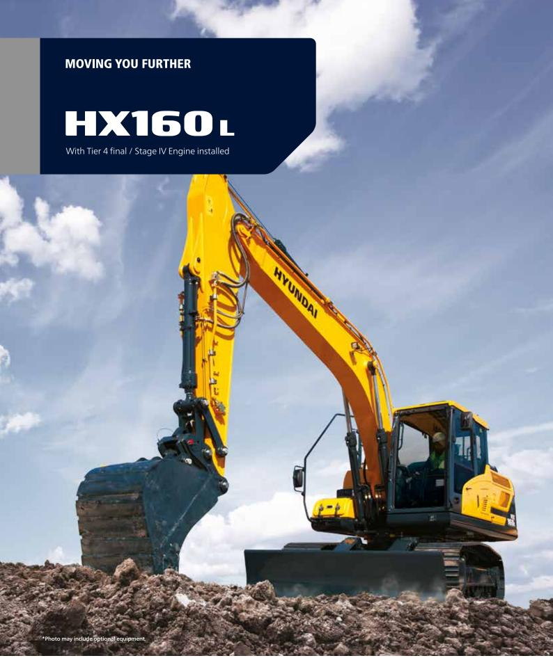
**Net Power** SAE J1349 / 96 kW (128 HP) at 2,050 rpm
